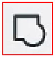
Group multiple shapes together by clicking this button. Subtraction occurs when grouping solid and hole; and one solid is combined when grouping two solids.
